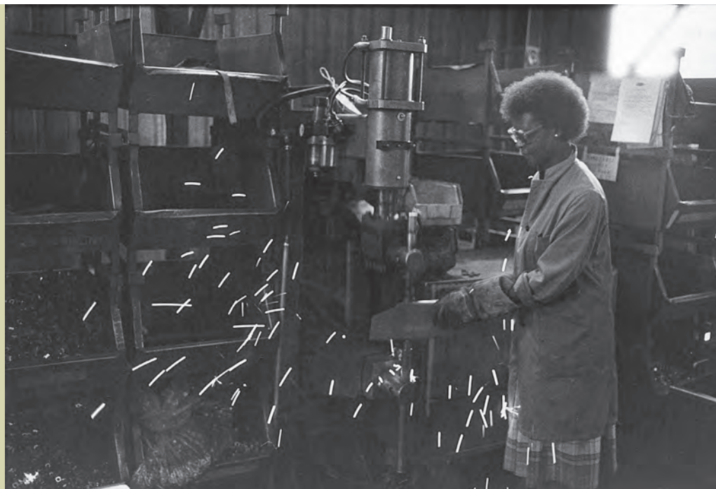
A WOMAN WORKER DOING PEDESTAL WELDING AT SAMCOL. Photo by Lesley Lawson, Taffy Adler Papers, AH2065/J 158
