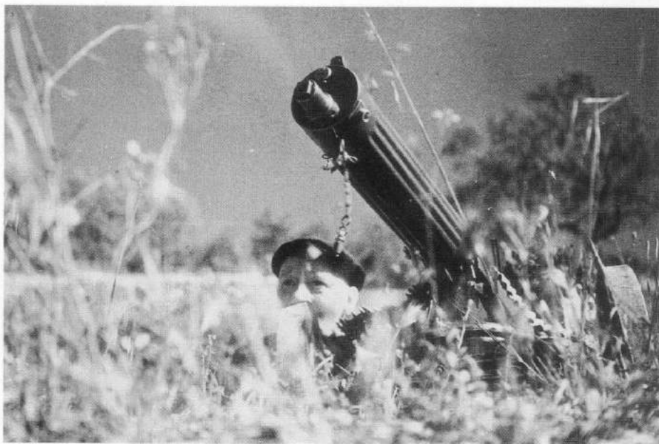
Maxim machine gun: many of those in the International Brigades were elderly M1910 Soviet models. In Spain they often had to be carried on the back; the two steel wheels of the carriage played havoc with the carrier's kidneys. (IBMA)
